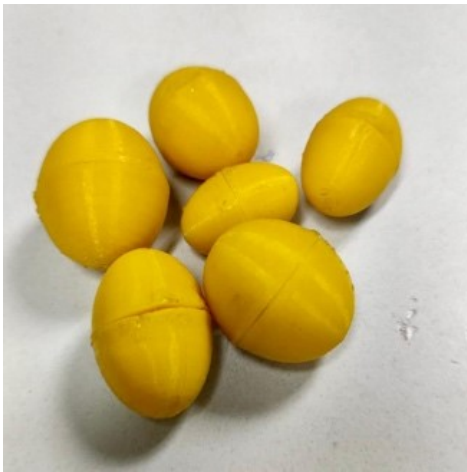
Fig. 2: Melon prototypes manufactured by using 3D printing technology.
